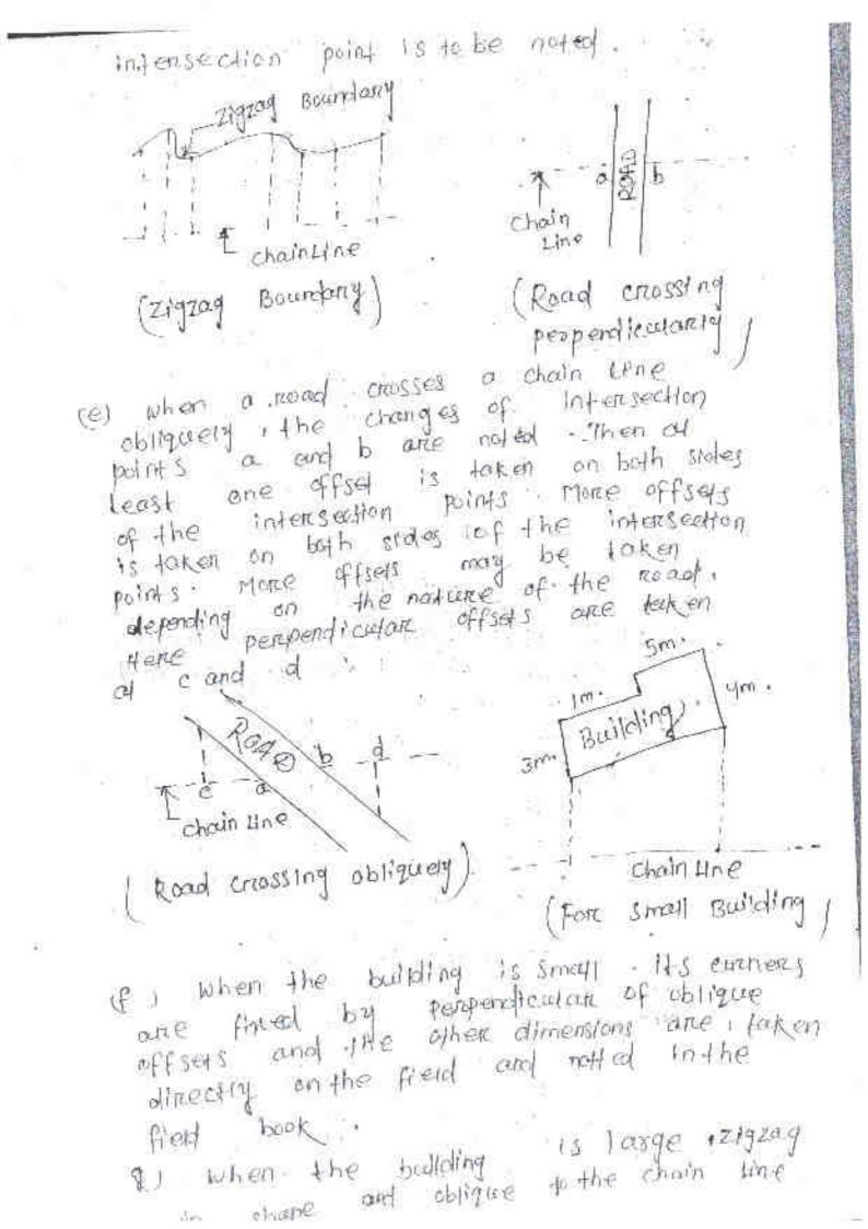
then the comments and flowed by perpendicular on oblique offsels. Then the full flan. of the buildings is alrawn on a separate page along with all the dimensions. This page should be attached with the fleid book of the proper place.
