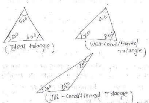
gul-conditioned tolongies are not used in their chain surveying - This is because their chain surveying one not sharp and well apex points are not sharp and well apex points are usight displacement defined, which is what excluse considerable of these points mainly course considerable enror in picting.
