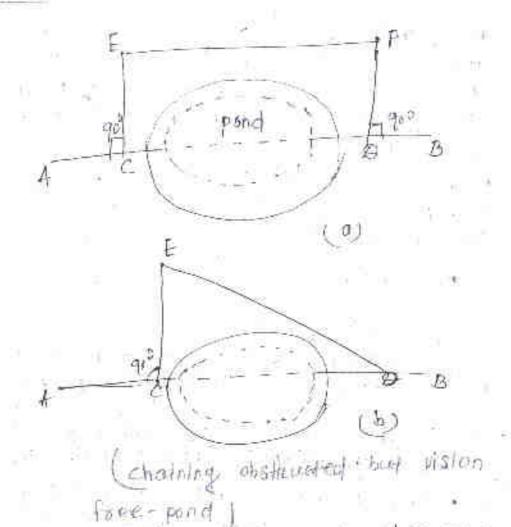
suppose AB is the chain line Two points e and D are selected on it on spostle banks of the pond. Equal perpendications ce and DF are exected at perpendications ce and DF are exected.
